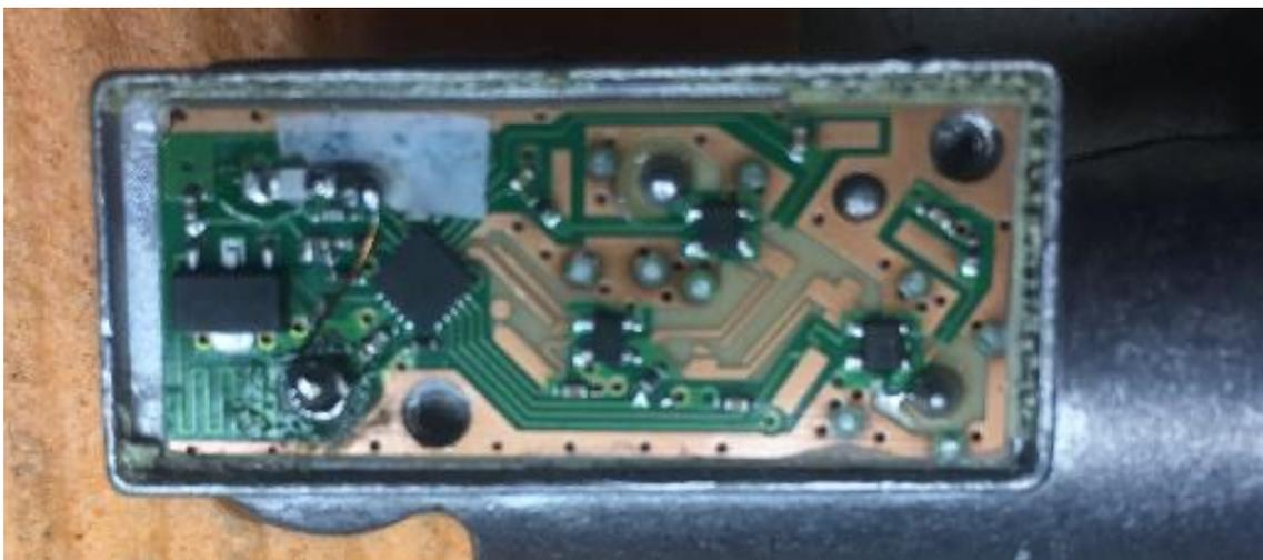
At the end it ends up like this! I put some paper tape underneath the series circuit the make soldering more easy. The parallel circuit is hardly visible around the centre pin.
