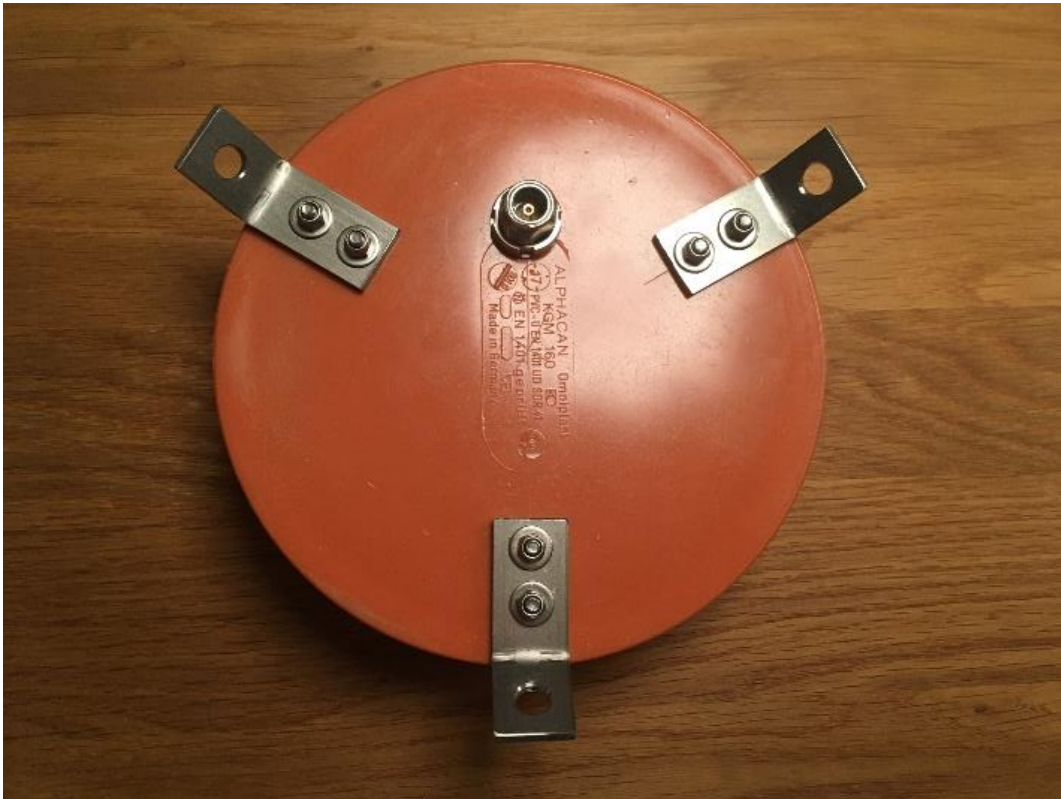
Backside of the feed with the dish mounting.
