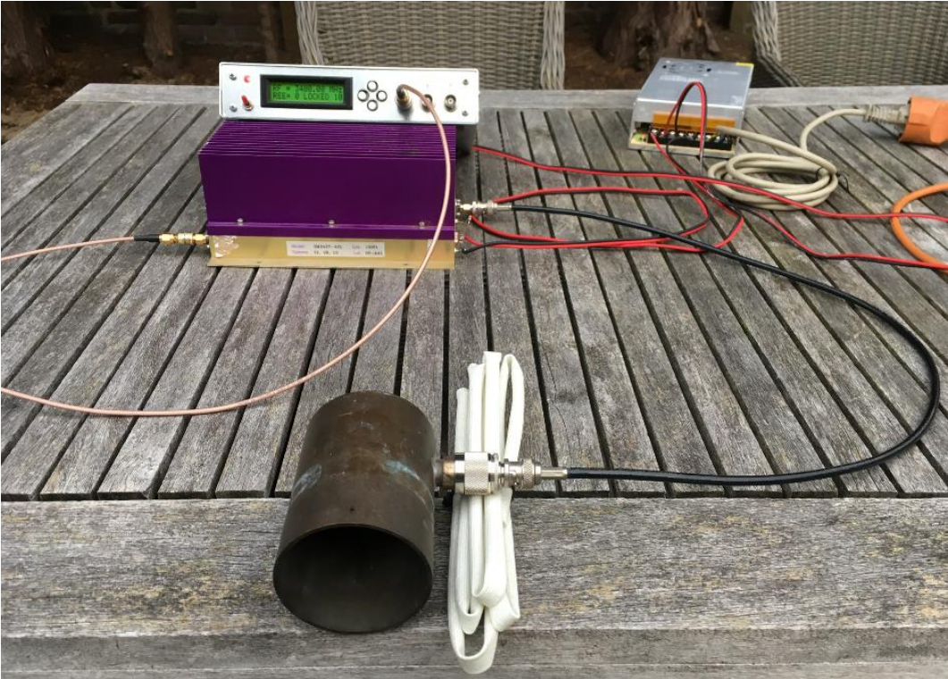
Signal source in the back of the garden to evaluate the antenna pattern. (9cm)
